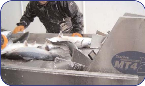
The 1990s saw the development of automated systems, mechanising the stunning operation and potentially making it a more consistently humane procedure. The operator gently grasps the fish near the middle of the body (not by the tail), guiding it into the opening of the machine to ensure the fish is upright. The fish activates the trigger system, resulting in the piston striking the fish on the head rendering it immediately unconscious.
