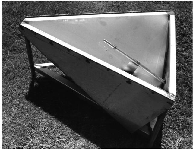
Figure 3. Inclined stainless steel pressure rinse/drain rack.
