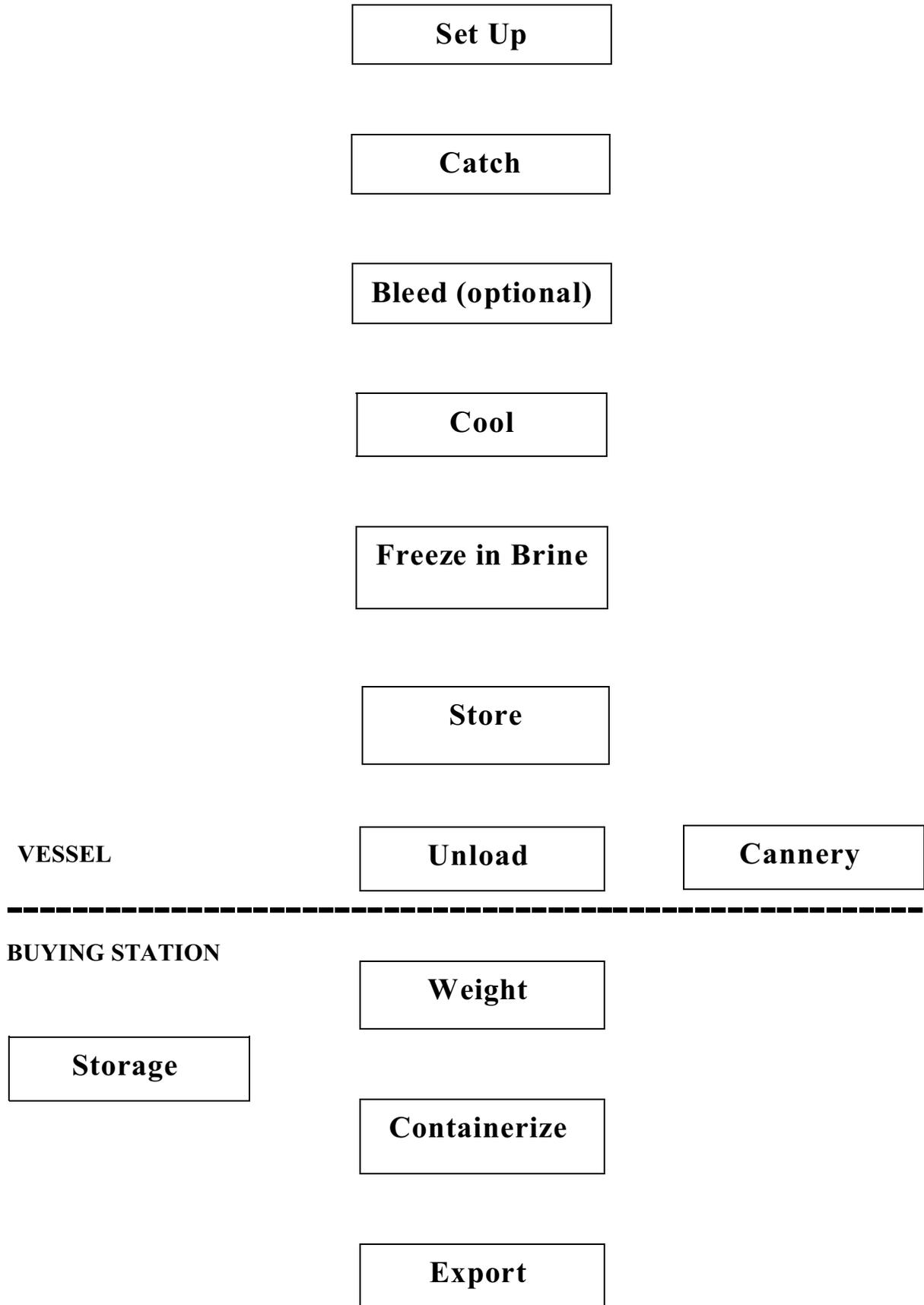
**BLAST PROCESS FLOW DIAGRAM**
